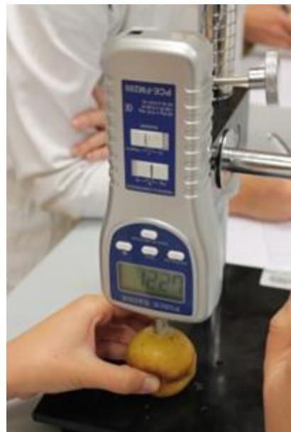
Slika 26. Digitalni stolni penetrometar (PCE-PT200, PCE Instruments, Southampton, UK)
