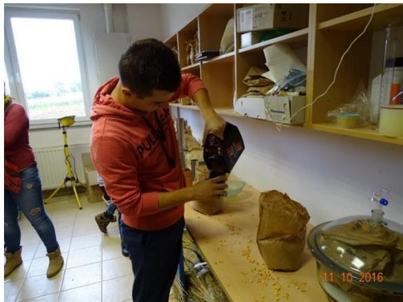
Slika 13. Mjerenje vlage aparatom Dickey John
